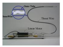
Fig. 5. Schematic diagram of flexible actuation system
