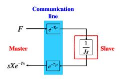
Fig. 7. Example of time delayed telehaptics system
